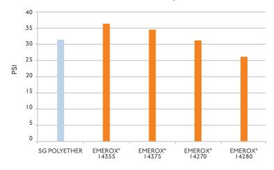
EMEROX® Polyols demonstrate excellent compression strength and dimensional stability properties compared to SG polyether.
