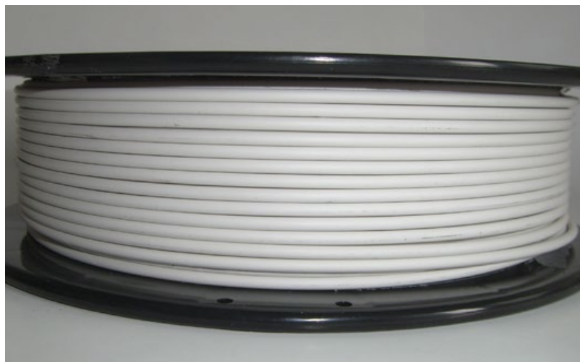
Fig. 3 A spool with aluminium oxide filament, 2.85 mm thickness
