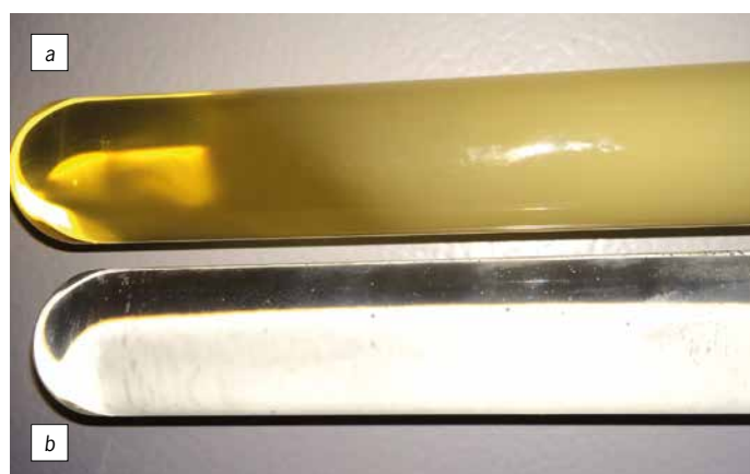
◀ Fig. 2: (a) Emerox 14060 + 4 pphp water; (b) adipate diethylene glycol + 4 pphp water
