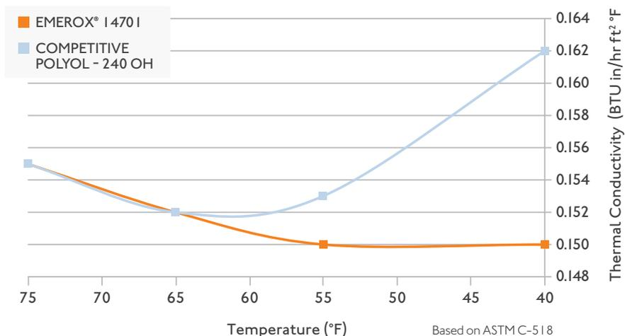
EMEROX® I 470 I offers improved low temperature thermal conductivity compared to a typical competitive polyol.
